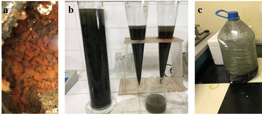
Figure 3.6 Different sludge used to inoculate the reactor. (a) Anammox sludge from the Anammox reactor (b) AD sludge (c) Sediment from Eymir Lake
